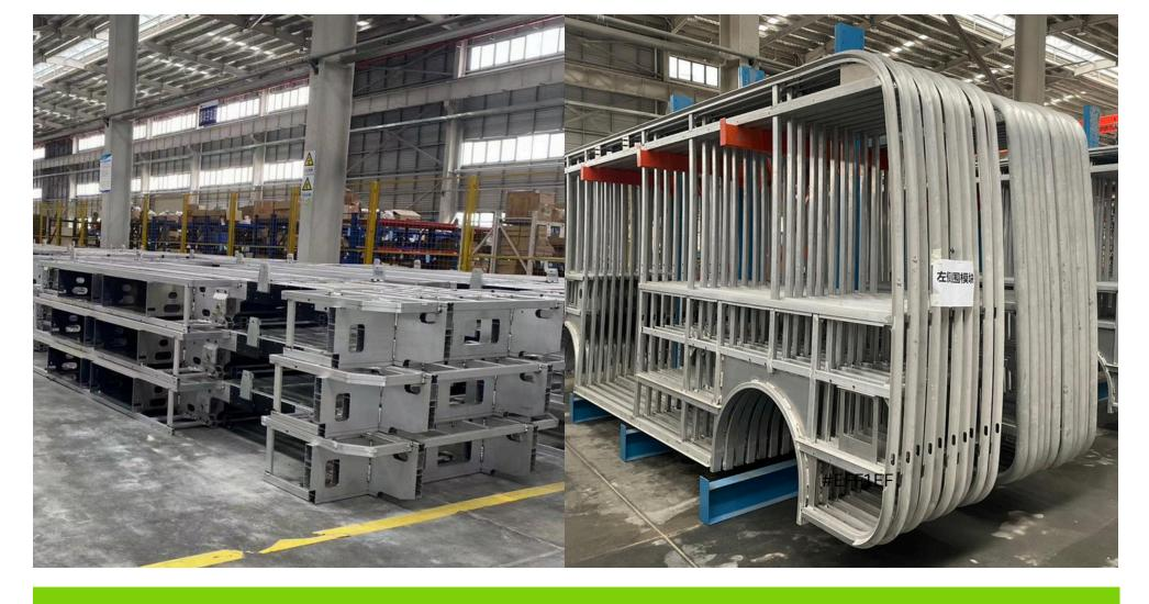
With a full aluminum monocoque body frame, we achieve a 40% reduction in weight and corrosion-free durability. Our warranty extends up to 10 years, reflecting our high confidence in the material aspect.
