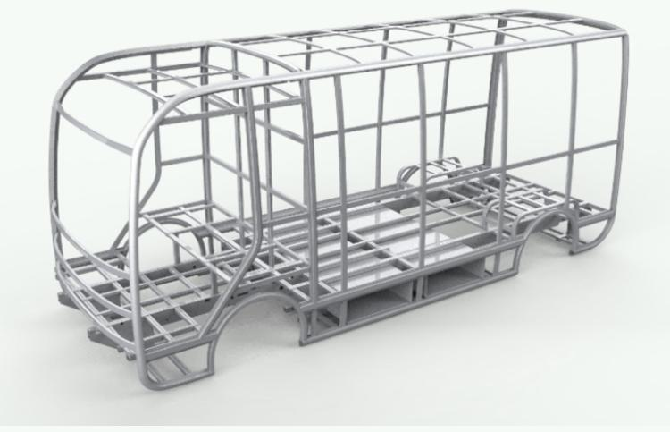
With a full aluminum monocoque body frame, we achieve a 40% reduction in weight and corrosion-free durability. Our warranty extends up to 10 years, reflecting our high confidence in the material aspect.
