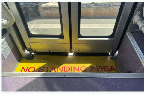
The electric folding door of designed bus the is provide convenient access while for passengers ensuring safety and efficiency during boarding and alighting.
