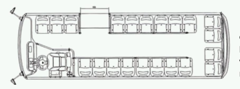
Customizing the seat arrangement by maximizing the seating capacity with 9 standee to fulfil customer's needs.
