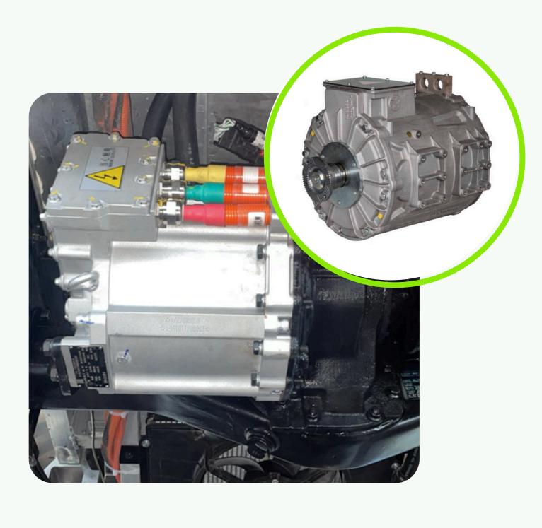
Inovance TZ210 electric motor has a power range of 60-120kW, operating at the torque between 290-480V. Besides that, it can travel up to 200km with AirCon ON and in a full load passengers condition
